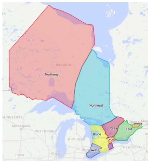
Ontario is divided into ten electricity zones defined by major interfaces (bulk transmission). IESO calculates nodal prices for reference nodes (i.e., buses) in each of the zones. Zones have different mix of generation assets. Several zones have more assets than peak demand. IESO is moving towards a system of Locational Marginal Prices (LMP).
